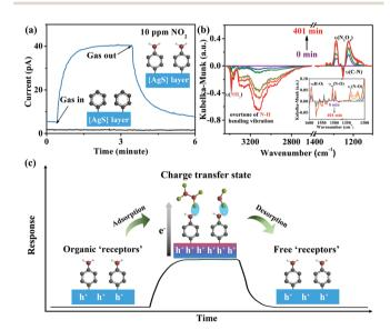
Fig. 4 (a) Response-recovery curves of Ag(SPh-NH<sub>2</sub>) (blue) and Ag(SPh) (black) to 10 ppm NO<sub>2</sub>. (b) In situ DRIFT Spectra for Ag(SPh-NH<sub>2</sub>) exposed to NO2 as a function of time. (c) Possible NO2 sensing mechanism for Ag(SPh-NH<sub>2</sub>).
