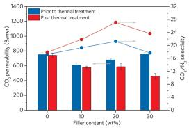
Fig. 5 Gas separation performance of the pure and composite membranes containing up to 30 wt% of MOF fillers. Both membranes before thermal treatment (blue) and after thermal treatment (red) are presented.
