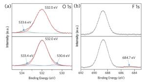
Fig. 4 XPS spectra for  $(ZIF-62)_{0.2}(6FDA-DAM)_{0.8}$  (top) and  $(a_gZIF-62)_{0.2}(6FDA-DAM)_{0.8}$ 62)<sub>0.1</sub>(6FDA-DAM)<sub>0.8</sub> (bottom), (a): O 1s, (b): F 1s.
