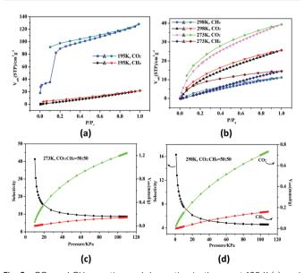
Fig. 2 CO<sub>2</sub> and CH<sub>4</sub> sorption and desorption isotherms at 195 K (a), and 273 and 298 K (b). The selectivity of  $\bf 2a$  for  $CO_2$  and  $CH_4$  (1:1) at 273 K (c) and 298 K (d), respectively
