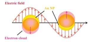
Fig. 1 Schematic illustration of the origin of LSPR.
