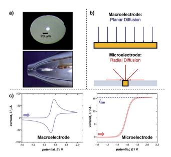
Fig. 18 (a) Optical microscope images of the top and side of an exemplar microelectrode. (b) The difference in transport to a macro-and microelectrode results in differing voltammetric responses, shown for a representative reversible oxidation in (c). Arrows in (c) demonstrate the direction of the scan, positive current represents oxidation. (a) Adapted with permission from ref. 65c. Copyright 2006 Institute of Physics Publishing.
