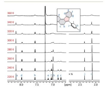
Fig. 4 Temperature-dependent  $^1H$  NMR spectra of **2** (CDCl<sub>3</sub>, 600 MHz). The signals were assigned at 220 K using 2D spectroscopic methods (see the ESI†).
