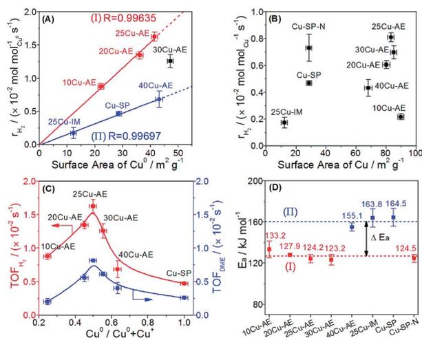
Fig. 4 Correlation of the H<sub>2</sub> production rate based on Cu<sup>0</sup> sites or total Cu sites with (A) the surface area of Cu<sup>0</sup> and (B) total surface area of Cu; (C) correlation of the TOF of H<sub>2</sub> and DME with the Cu<sup>0</sup>/(Cu<sup>0</sup> + Cu<sup>+</sup>) ratio; (D) apparent activation energies of the catalysts.
