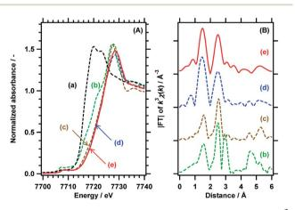
Fig. 2 (A) Co-K edge XANES data and (B) Fourier transforms of  $k^3$ weighted Co-K EXAFS spectra for (a) CoCl<sub>2</sub>·6H<sub>2</sub>O, (b) Co<sub>3</sub>O<sub>4</sub>, (c) CoOOH, and RhCrO<sub>x</sub>/SrTiO<sub>3</sub>:Al coloaded with 0.3 wt% Co species (d) in darkness and (e) following UV illumination for 15 h by a 300 W Xe lamp.
