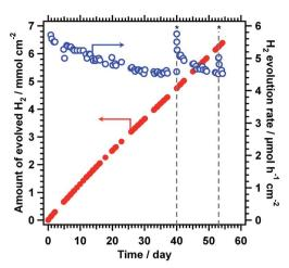
Fig. 4 Time course of water splitting activity of  $5 \times 5 \text{ cm}^2 \text{ TiO}_2/\text{CoOOH/RhCrO}_x/\text{SrTiO}_3$ :Al sheet in panel reactor. Reaction conditions: photocatalyst, 20 mg; reaction solution, 1 mm deep distilled water; reaction temperature, 291 K; light source, AM 1.5G solar simulator. Asterisk symbols (\*) indicate interruption of the illumination for two days.
