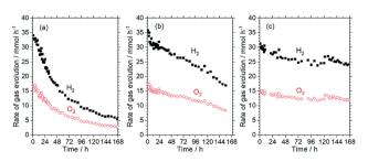
Fig. 1 Time courses of water-splitting activity of  $SrTiO_3$ :Al loaded with (a)  $RhCrO_x$ , (b)  $RhCrO_x$  and 0.3 wt% Co species, and (c)  $RhCrO_x$ , 0.3 wt% Co species and 3 wt%  $TiO_2$ . Reaction conditions: photocatalyst, 0.5 g; reaction solution, 370 mL distilled water; reaction temperature, 291 K; light source, 450 W high-pressure Hg lamp ( $\lambda > 300$  nm).
