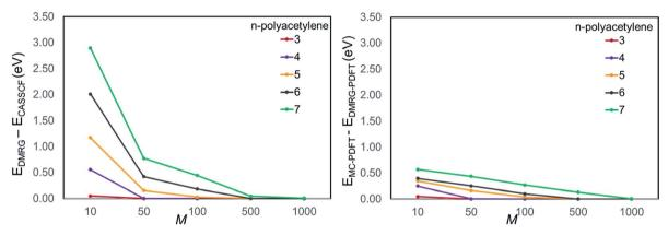
Fig. 3 Convergence of (a) DMRG and (b) DMRG-PDFT with respect to conventional CASSCF and MC-PDFT, respectively. The ordinate is the mean of the difference between (a) conventional CASSCF and DMRG energies and (b) conventional MC-PDFT and DMRG-PDFT energies for singlet and triplet states.
