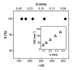
Fig. 10 1-Hexene conversion (X) versus bubble residence time ( $\tau$ ) in scaled-up mesoreactor. Insert shows the turnover frequency of the reactor at different flow velocities. Turnover frequency is defined as number of moles of 1-hexene converted to product per number of moles of catalyst per unit time.
