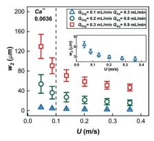
Fig. 8 The thickness of the annular film around the gas bubbles estimated by fitting the mathematical model of egn (3) at different volumetric liquid flow rates and bubble speeds. Insert shows a magnified view of the thickness of the annular film for  $Q_{Org} = 0.1 \text{ mL}$  $min^{-1}$ ,  $Q_{Aq} = 0.3 \text{ mL min}^{-1}$ . (for Ca\*\* see ESI† section 1).
