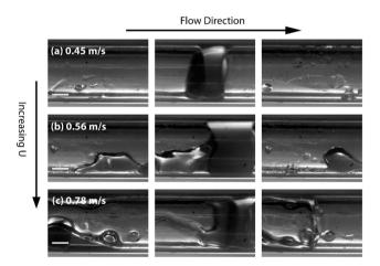
Fig. 4 (a)-(c) High-speed stereomicroscope images at higher flow velocities in 2 m long 3.2 mm ID PTFE channel, highlighting the extent of droplet breakup with increasing flow speed.  $Q_{\rm Org}$  = 0.1 mL min<sup>-1</sup>,  $Q_{\rm Aq}$  = 0.3 mL min<sup>-1</sup>,  $Q_{\rm Gas}$  = 115 mL min<sup>-1</sup>, 120 mL min<sup>-1</sup> and 146 mL min<sup>-1</sup> respectively. All scale bars represent 1 mm.
