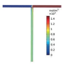
Fig. 3 Three dimensional CFD mixing, without reaction, of 1.5 mol m<sup>-3</sup> of both M4MAA (1) and DMF-DMA (2) entering a tee junction from left and right respectively and exit mixed downward. Pé and Re numbers for this simulation are  $1.51 \times 10^5$  and 5.02 respectively. Red and blue indicate high and low concentrations of DMF-DMA (2) respectively. The dashed line indicates where the reaction was assumed to initiate due to removal of the tee junction.
