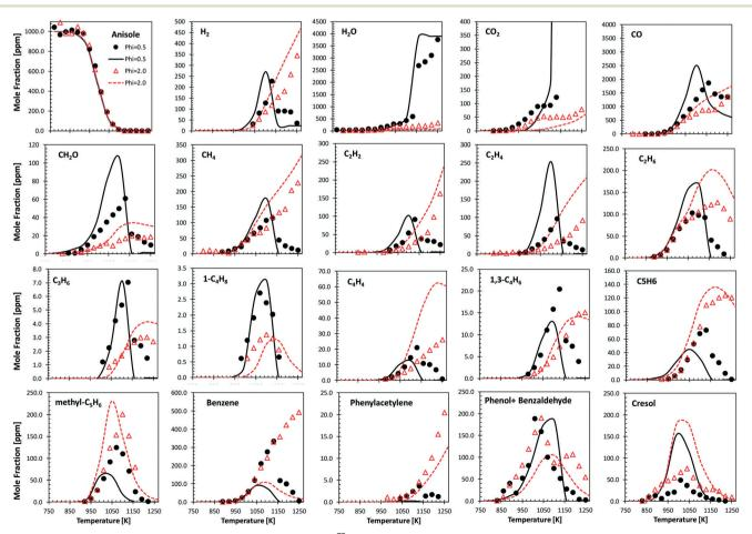
Fig. 9 Anisole atmospheric pressure oxidation in an Orleans JSR. 5 0.1% anisole/ $O_2/N_2$  mixtures under rich ( $\varphi = 2.0$ , triangles) and lean conditions  $(\varphi = 0.5, \text{ circles})$ . Comparisons between experimental data (symbols) and model predictions (lines).
