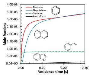
Fig. 18 Vanillin pyrolysis. Successive formation of benzene, styrene, naphthalene, and benzofuran, at 1073 K.
