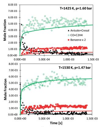
Fig. 10 Measured (symbols)<sup>76</sup> and simulated (lines) species profiles of main species during the shock-tube pyrolysis of 0.5% anisole, 1% Ar in
