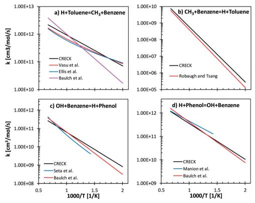
Fig. 7 Comparisons between the proposed rate rules for ipso-addition reactions and literature values. Panels a) and b): H + toluene = CH<sub>3</sub> +  $C_6H_6$ , forward and backward. Panels c) and d): OH + benzene = H + phenol, forward and backward.
