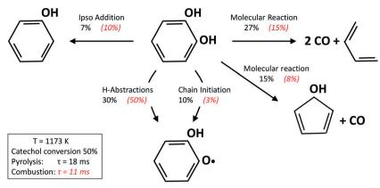
Fig. 13 Catechol pyrolysis and oxidation at p = 1 atm and 1173 K. Reaction flux analysis
