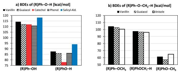
Fig. 4 Comparison of vanillin BDEs [kcal mol<sup>-1</sup>] with respect to different aromatic compounds. Panel a) hydroxyl group; panel b) methoxy group.
