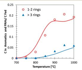
Fig. 14 Carbon (C) in 1-2 ring aromatics and heavier PAHs from catechol pyrolysis at p = 1 atm and  $\tau = 0.3$  s. Comparison between model predictions (lines) and experimental data (symbols with dashed lines).4
