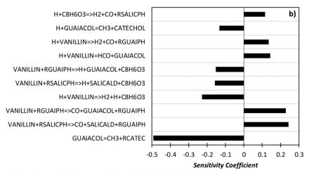
Fig. 17 Sensitivity analysis of phenol (panel a) and guaiacol (panel b) at 973 K and 50% vanillin conversion.
