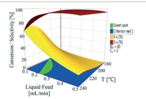
Fig. 8 Sweet spot plot based on objectives of >40% conversion and >99% selectivity in single-pass mode for varying temperature (180-240 °C) and liquid feed flow (0.1–0.5 mL min<sup>-1</sup>, 0.7–3.3 m<sup>3</sup> m<sup>-2</sup> h<sup>-1</sup> at STP) at fixed nitrogen flow (40 mL min<sup>-1</sup>, 266.4 m<sup>3</sup> m<sup>-2</sup> h<sup>-1</sup> at STP) and substrate concentration (5 wt%).
