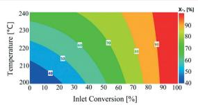
Fig. 7 Influence of reactor inlet conversion (0-100%) and temperature (200-240 °C) on reactor outlet conversion in recycle mode with substrate concentration of 5 wt% and nitrogen flow of 45 mL min<sup>-1</sup> (299.7 m<sup>3</sup> m<sup>-2</sup> h<sup>-1</sup> at STP).
