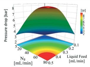
Fig. 5 Influence of nitrogen flow (5–80 mL  $\min^{-1}$ , 33.3–566.7 m<sup>3</sup> m<sup>-2</sup>  $h^{-1}$  at STP) and liquid feed flow (0.1–0.5 mL min<sup>-1</sup>, 0.7–3.3 m<sup>3</sup> m<sup>-2</sup>  $h^{-1}$ at STP) on the pressure drop for a substrate concentration of 1 wt% at 220 °C, in single-pass mode.
