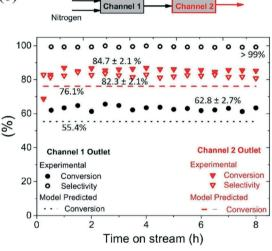
Fig. 6 Influence of intermediate gas (nitrogen and hydrogen) on selectivity for the dehydrogenation cyclohexanedionein two-channels-in-series in continuous mode (a) with intermediate hydrogen removal and (b) without hydrogen removal.
