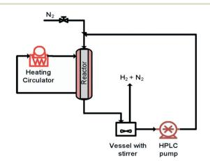
Fig. 10 The simplified scheme of semi-continuous dehydrogenation (recycle mode) of 1,4-cyclohexanedione.
