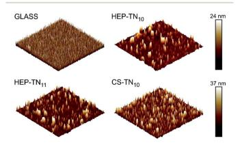
Fig. 4 Representative 10  $\mu m \times 10 \mu m$  AFM topographic images of the glass (non-modified), CS-TN $_{10}$ , HEP-TN $_{10}$  and HEP-TN $_{11}$  surfaces.
