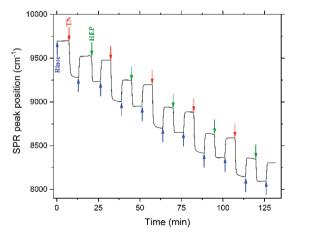
Fig. 2 PEM assembly monitored by in situ FT-SPR. Arrows represent the beginning of acidified water rinse (blue), TN deposition layers (red), and HEP deposition layers (green).
