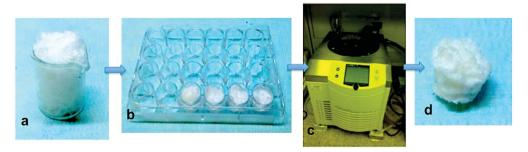
Fig. 1 Schematic representation of the fabrication method: the polymeric foam was obtained from the gas foaming process during which the generated carbon dioxide is incorporated into the polymer (a). The PVA foam was poured in a mold (b), frozen at -20 °C for 6 h, freeze-dried for a 24 h, (c) and then the scaffolds were extracted from the mold (d).
