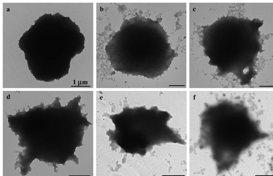
Fig. 2 TEM images showing the process of the protrusion of nanopikes on the surface of CSEG-*g*-Chol MGs after being incubated in a glutathione solution (5 mM) for 0 (a), 0.5 (b), 1 (c), 3 (d), 12 (e) and 24 h (f), respectively.
