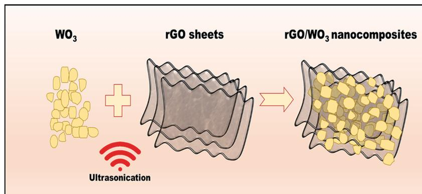
Fig. 1 Schematic representation of rGO/WO<sub>3</sub> nanocomposite formation using the ultrasonication method.
