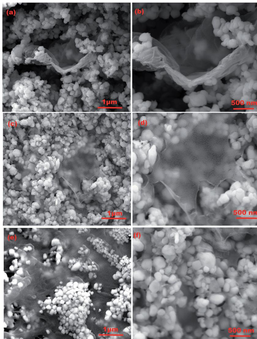
Fig. 4 FESEM images of different weight percentages of rGO/WO<sub>3</sub> nanocomposites (1%, 5% and 10%): (a and b) 1% rGO/WO<sub>3</sub>, (c and d) 5% rGO/WO<sub>3</sub>, and (e and f) 10% rGO/WO<sub>3</sub>. (f) EDAX analysis of rGO/WO<sub>3</sub> nanocomposites.
