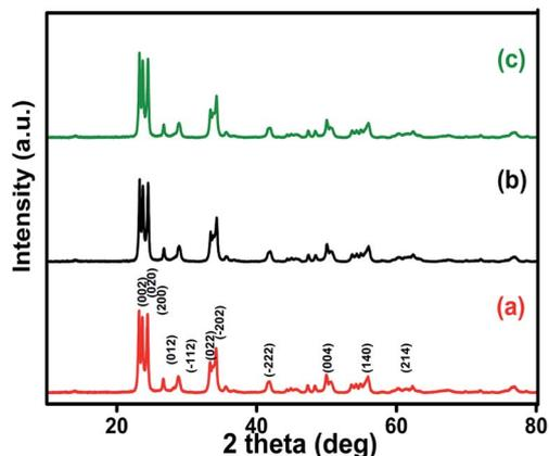
Fig. 2 Powder XRD spectra of different weight percentages of 1%, 5% and 10% rGO/WO<sub>3</sub> nanocomposites: (a) 1% rGO/WO<sub>3</sub>, (b) 5% rGO/WO<sub>3</sub> and (c) 10% rGO/WO<sub>3</sub>.
