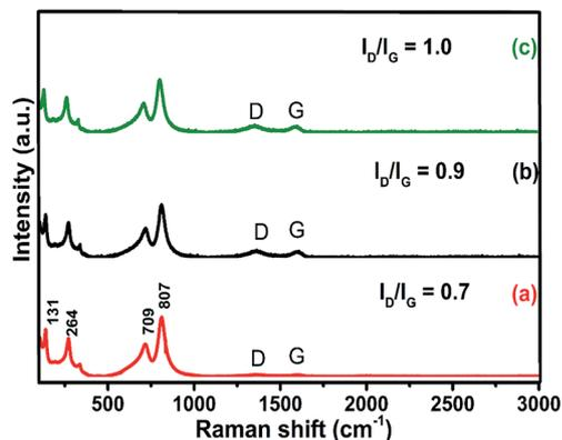
Fig. 3 Raman spectra of different weight percentages of nanocomposites (1%, 5% and 10% rGO/WO<sub>3</sub>): (a) 1% rGO/WO<sub>3</sub>, (b) 5% rGO/WO<sub>3</sub> and (c) 10% rGO/WO<sub>3</sub>.
