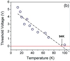
Fig. 4 (a) Temperature dependent I-V plots of the sensor in the bias range from -20 V to +20 V. (b) Threshold voltage ( $V_{Th}$ ) as a function of temperature.
