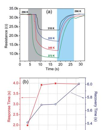
Fig. 8 (a) Sensor response at different temperatures in the  $296-373 \, \text{K}$  temperature range, and (b) response and recovery time of the sensor at the corresponding temperatures.
