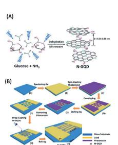
Fig. 11 Use of glucose-derived QDs for the fabrication of photodetectors. This figure has been adapted/reproduced from ref. 166 with permission from the American Chemical Society.
