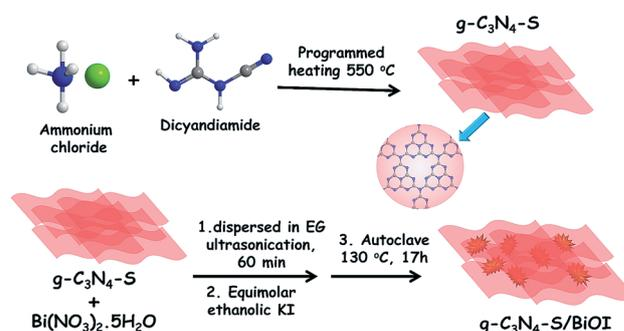
Fig. 1 Synthetic strategy of  $g\text{-C}_3\text{N}_4\text{-S}/\text{BiOI}$  heterojunction composite.
