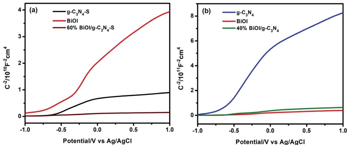
Fig. 6 Mott–Schottky plots for (a) pristine  $g\text{-C}_3\text{N}_4\text{-S}$ , pristine BiOI and  $g\text{-C}_3\text{N}_4\text{-S/BiOI}$  and (b) pristine  $g\text{-C}_3\text{N}_4$ , pristine BiOI and  $g\text{-C}_3\text{N}_4\text{/BiOI}$ . The plots are shown in two different figures with two different scales (vertical axis) for improved visibility.
