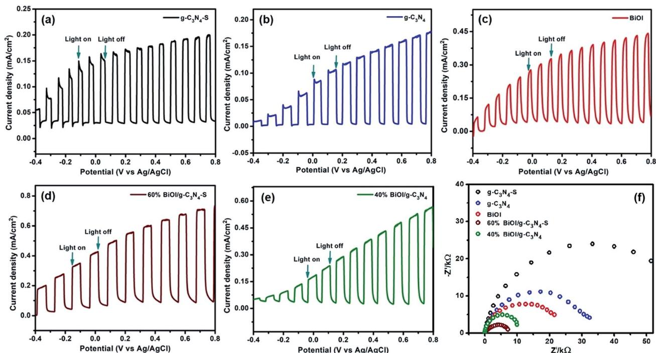
Fig. 5 Light on–off experiment for (a) pristine  $g\text{-C}_3\text{N}_4\text{-S}$  (b) pristine  $g\text{-C}_3\text{N}_4$  (c) pristine BiOI (d)  $g\text{-C}_3\text{N}_4\text{-S}/\text{BiOI}$  and (e)  $g\text{-C}_3\text{N}_4/\text{BiOI}$ ; (f) Nyquist plots for the investigated samples obtained from EIS.
