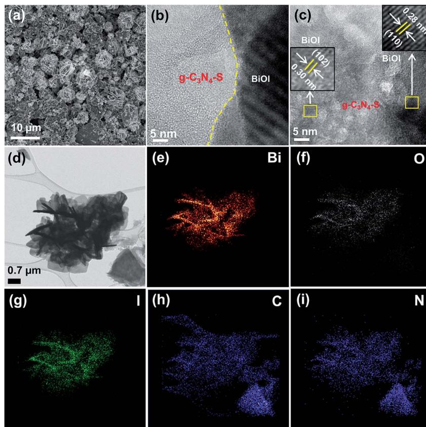
Fig. 2 (a) FESEM image of  $g\text{-C}_3\text{N}_4\text{-S}/\text{BiOI}$  thin film (b) HRTEM image showing heterojunction of BiOI and  $g\text{-C}_3\text{N}_4\text{-S}$  (c) HRTEM image showing lattice fringes (and insets showing  $d$ -spacing) corresponding to  $g\text{-C}_3\text{N}_4\text{-S}$  and BiOI (d) bright field STEM image of  $g\text{-C}_3\text{N}_4\text{-S}/\text{BiOI}$ ; STEM elemental mapping for (e) Bi, (f) O, (g) I, (h) C and (i) N.
