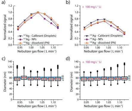
Fig. 3 (a) Normalised signal intensities recorded for Ag analyte in the form of NPs, microdroplets and enriched  $^{109}$ Ag solution without any additional matrix at nebulizer gas flow rates between 0.94 and 1.12 L min $^{-1}$ . (b) Same experiment as in (a), but with 100 mg L $^{-1}$  Li matrix. (c) and (d) Corresponding sizing of the 80 nm Ag NPs at different nebulizer gas flow rates. In both (c) and (d), the shaded blue area shows the expected NP diameter from the manufacturer.
