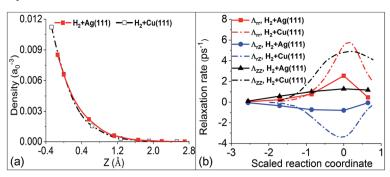
Fig. 3 (a) Comparison of the clean metal substrate electron density evaluated at the position of an H atom moving along the MEPs for dissociation on Cu(111) and Ag(111), as a function of the relative height with respect to the molecular center at the transition state (i.e.  $Z_{TS} = 0$ ). (b) Comparison of the mode-specific electronic friction computed by TDPT along the MEPs for H<sub>2</sub> dissociation on Cu(111) and Ag(111).
