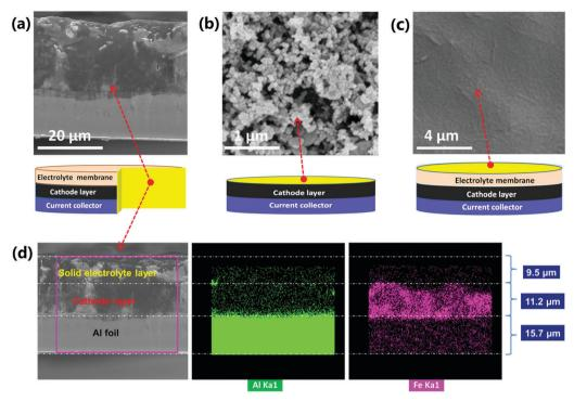
Fig. 3 (a) SEM image of the cross section of the cathode-supported PPAL solid electrolyte membrane. (b) Surface morphology of the LiFePO₄ cathode layer. (c) Surface morphology of the PPAL solid electrolyte membrane. (d) EDS maps of Al and Fe in the cross section of the cathode-supported PPAL solid electrolyte membrane
