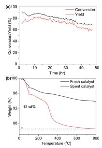
Fig. 6 (a) Stability test for Ni/Al $_2$ O $_3$ -PD catalyst.1-Hexanol at 1  $\mu$ L min $^{-1}$  with 8 mL min $^{-1}$  NH $_3$  and 20 mL min $^{-1}$  N $_2$  flowed through 200 mg catalyst at 230 °C. GHSV = 1.12 × 10 $^4$  h $^{-1}$ . (b) TG analysis for Ni/Al $_2$ O $_3$ -DP catalyst before and after reaction.
