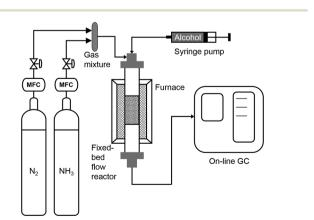
Scheme 1 Experimental set-up for the conversion of alcohols to
