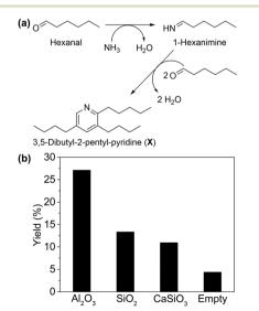
Fig. 1 (a) Scheme for formation of 3,5-dibutyl-2-pentyl-pyridine (compound X) and (b) yield of compound X with different supports. Reaction conditions: 1  $\mu$ L min<sup>-1</sup> hexanal, 200 mg catalyst, 190 °C, 8 mL min<sup>-1</sup> NH<sub>3</sub>, 20 mL min<sup>-1</sup> N<sub>2</sub>. GHSV = 1.12 × 10<sup>4</sup> h<sup>-1</sup>.
