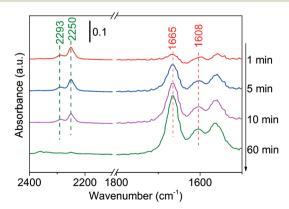
Fig. 5 DRIFTS of adsorbed butanenitrile on Ni/Al<sub>2</sub>O<sub>3</sub>-DP surface as a function of time under  $N_2$  flow at 100 °C. At t = 0 min, butanenitrile
