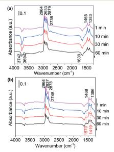
Fig. 3 DRIFTS of adsorbed species on (a) Al<sub>2</sub>O<sub>3</sub> surface and (b) Ni/  $Al_2O_3$ -DP surface as a function of time under  $N_2$  flow at 130 °C. At t =0 min, 1-butanol was injected.
