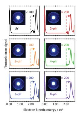
Fig. 3 Two-photon resonance-enhanced photoelectron spectra of phenolate and para-substituted alkyl-phenolate anions recorded at photon energies that are resonant with a DBS (see Fig. 2(a)). The signal has been amplified at higher electron kinetic energies (>2.0 eV) for clarity. Inset are the raw photoelectron images from which the spectra have been extracted. The central feature has been intentionally saturated to emphasise the outer narrow and anisotropic ring.
