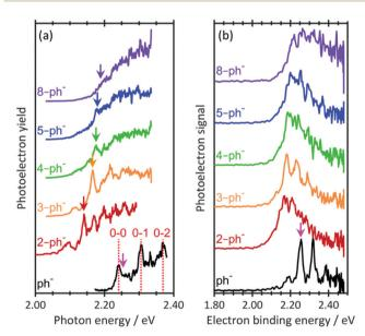
Fig. 2 (a) Photodetachment action spectra for n = 0, 2–5, and 8 near the photodetachment threshold. Vertical lines dashed lines indicate transitions measured by Liu et al.44 Vertical arrows indicate excitation energy for resonance-enhanced photoelectron spectra in Fig. 3. (b) Photoelectron spectra of phenolate and para-substituted alkyl-phenolate anions at hv = 2.48 eV. All spectra have been vertically offset for clarity. The electron affinity (EA) is indicated by the vertical pink arrow
