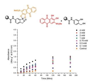
Fig. 2 UV-Vis absorption per gram of **BOB** upon addition of various concentrations of  $H_2O_2$  (0–4 mM) in PBS (pH 7.4, PBS = 0.01 M) over time (minutes). Absorbance was measured at 513 nm at 25 °C. Error bars indicate standard deviation (n = 3).
