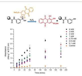
**Fig. 1** UV-Vis absorption per gram of **PBA** upon addition of various concentrations of  $H_2O_2$  (0–4 mM) in PBS (pH 7.4, PBS = 0.01 M) over time (minutes). Absorbance was measured at 513 nm at 25 °C. Error bars indicate standard deviation (n = 3).
