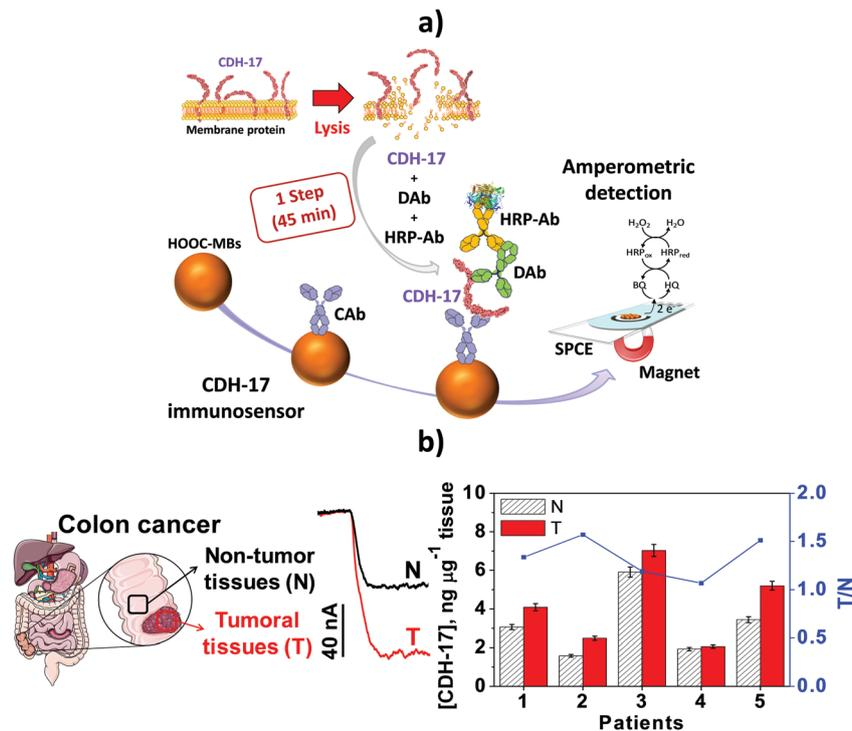
Fig. 15 (a) Schematic illustration of the immunosensor developed for CDH-17 determination. Illustrative examples of amperograms recorded with the immunosensor of 0.5  $\mu\text{g}$  of protein extracts obtained from a tumor (T) and paired healthy tissue (N), and CDH-17 concentrations obtained in the analyzed tissue extracts. Error bars are three times the standard deviation of three replicates. Reproduced and adapted from ref. 32 with permission.
