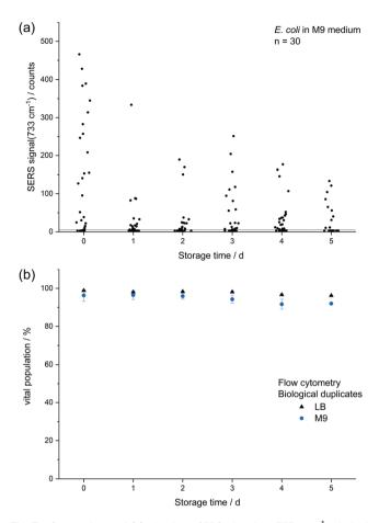
Fig. 3 Comparison of (a) absolute SERS signal at 733 cm<sup>-1</sup> of single E. coli cells which were cultured to the stationary phase and either directly subjected to in situ AgNP synthesis or first stored up to 5 d and (b) viability of E. coli measured by flow cytometry with two DNA intercalating dyes (propidium iodide: dead, SYTO 9: viable) after 0-5 d storage.
