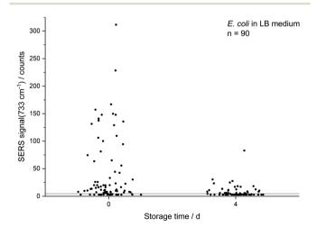
Fig. 2 Decreasing absolute SERS intensity at 733 cm<sup>-1</sup> of single *E. coli* (LB medium) cells which were cultured to the stationary phase and either directly subjected to in situ AgNP synthesis or first stored for 4 d. Values are scattered on the abscissa for better readability.
