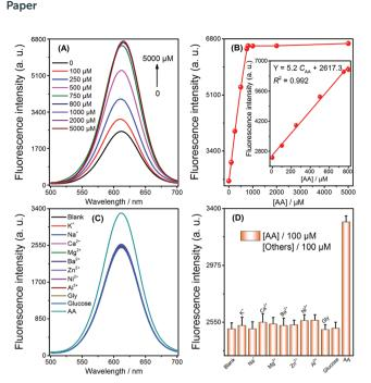
Fig. 2 The analytical performance and selectivity of this sensor for AA detection. (A) and (B) Fluorescence spectra and calibration curve for AA detection. Inset: A linear relationship of the fluorescence signal versus the concentration of AA ranging from 0 to 800  $\mu\text{M}$ . (C) and (D) Fluorescence spectra and fluorescence signal of different interferents. All concentrations were 100  $\mu\text{M}$ . Error bars were estimated from at least three replicate measurements.
