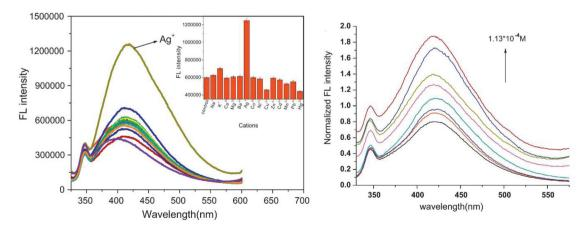
Fig. 2 Fluorescence emission spectra of FONs  $(7.5 \times 10^{-6} \text{ M})$  with or without various cations and plot of the fluorescent intensity as a function of Ag<sup>+</sup> concentration. Adapted with permission from ref. 46. Copyright 2011 Elsevier Ltd.
