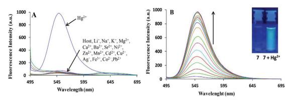
Fig. 13 (A) Changes in the fluorescence emission spectra of 195 nM solution of 12 (FON) upon the addition of 10  $\mu$ M of different metal ion salts in 15 aqueous media; (B) changes in the fluorescence emission spectra of 195 nM solution of 12 (FON) upon the successive addition of 0 to 10  $\mu$ M of Hg<sup>2+</sup> in an aqueous medium. Adapted with permission from ref. 70. Copyright 2013 the Centre National de la Recherche Scientifique (CNRS) and the Royal Society of Chemistry.
