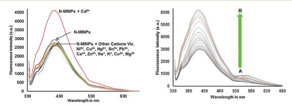
Fig. 11 Selectivity of 11 toward  $Cd^{2+}$  shows fluorescence enhancement as compared to other cations, and the fluorescence spectra of *N*-MINP suspension (1 × 10<sup>-5</sup> M) in the presence of different concentrations of  $Cd^{2+}$  ions. Adapted with permission from ref. 69. Copyright 2015 Elsevier Ltd.
