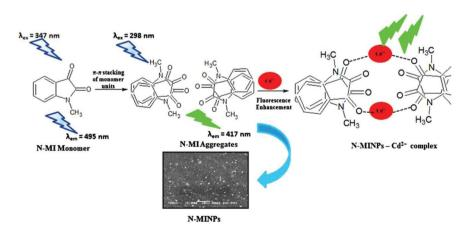
Fig. 12 Proposed graphic for the formation of 11 and its complexation with Cd<sup>2+</sup> ions. Adapted with permission from ref. 67. Copyright 2015 Elsevier Ltd.
