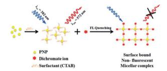
Fig. 6 Proposed mechanism for the formation of CTAB PNPs and surface-bound stable nonfluorescent micellar complexes with dichromate ions. Adapted with permission from ref. 60. Copyright 2014 the Royal Society of Chemistry.
