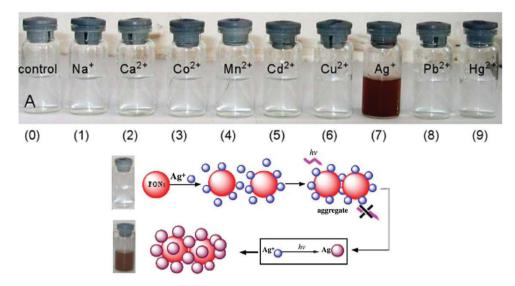
Fig. 3 Photographs of FON solutions after adding  $5 \times 10^{-4}$  M of the indicated metal ions after 24 h and the schematic illustration of the possible structure of Aq-nanoparticle-coated 3 aggregates. Adapted with permission from ref. 50. Copyright 2008 Elsevier Ltd.
