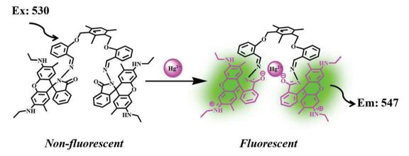
Fig. 14 Process of sensing through the coordination of Hg<sup>2+</sup>. Adapted with permission from ref. 70. Copyright 2013 CNRS and the Royal Society of Chemistry.
