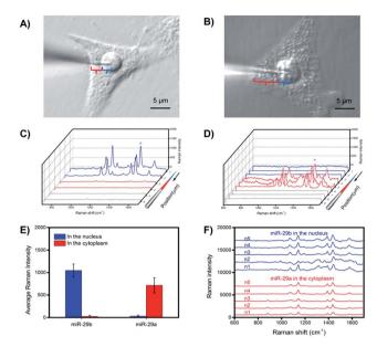
Fig. 6 An image showing the position of an extraction microprobe for probing (A) miR-29b and (B) miR-29a within a single HeLa cell. Raman spectra for (C) miR-29b and (D) miR-29a obtained along the extraction microprobe. (E) Average Raman intensity of miR-29b and miR-29a in single living HeLa cells with subcellular resolution. (F) Representative Raman spectra of multiple probe measurements of miR-29b and miR-29a in the nucleus and cytoplasm, respectively.
