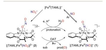
Scheme 2 Schematic representation showing the generation of [(TAML)Fe<sup>III</sup>(NO)]<sup>-</sup>.
