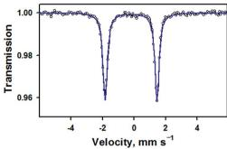
Fig. 2 Zero-field Mössbauer spectrum (black opened circles) and fit (blue line) of 1 measured at 77 K. The isomer shift of  $-0.19~\rm mm~s^{-1}$  and quadrupole splitting of 3.29 mm s<sup>-1</sup> are in good agreement with parameters previously reported for this complex in ref. 14 (also see Table S3, ESI†).
