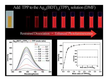
Fig. 4 PL variation trend of the Ag<sub>29</sub>(BDT)<sub>12</sub>(TPP)<sub>4</sub> NC resulting from the addition of different molar ratios of TPP ligand. (Top) PL intensity variation monitored by digital photography of the Ag<sub>29</sub>(BDT)<sub>12</sub>(TPP)<sub>4</sub> NC in the solution state under UV light. (Bottom-left) PL intensity variation monitored using the fluorescence spectrometer. (Bottom-right) PL intensity variation monitored at the fixed point of 642 nm.
