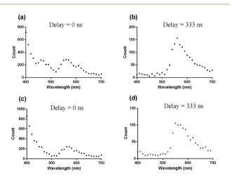
Fig. 1 Time-resolved fluorescence emission spectra of complex 13 in PBS buffer (pH = 7.0, 25  $^{\circ}$ C) in the presence of Cm-460 at (a) delay = 0 ns and (b) delay = 333 ns or with THS at (c) delay = 0 ns and (d) delay = 333 ns. The peak of complex 13 was partially obscured by the emission peaks of the fluorescent media when delay = 0 ns, while the peak of complex 13 became more evident when delay = 333 ns.
