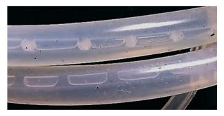
Fig. 5 Image of crystallisation tubing within the cooling tubing jacket at the beginning of the KRAIC. Lower tube is 0.3-0.5 m crystallisation length (32-28 °C), upper tube is 0.9-1.1 m (25-23 °C). N.B. crystals can be seen in solution slugs within the upper tubing.
