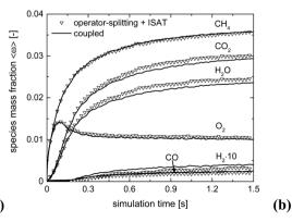
Fig. 5 Comparison of the average mass fraction composition for the isothermal CPO process, derived with: coupled approach and operatorsplitting (a) and coupled approach and operator-splitting + ISAT (b).
