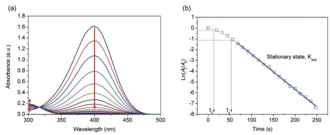
Fig. 12 Reduction of 4-nitrophenol by sodium borohydride by 2.24 × 10<sup>-5</sup> g L<sup>-1</sup> silver nanoparticles. (a) UV-vis absorption spectra of the solution as a function of time. (b) Kinetic analysis of the system after the induction period.
