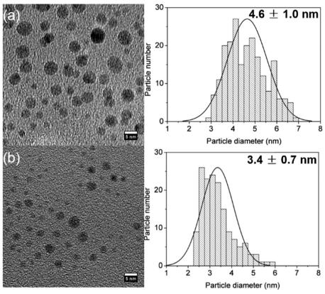
Fig. 5 Size and size distribution Ag nanoparticles from (a) SHR and (b) CFIR; helix diameter: 10 mm, pitch distance: 1/π cm, length: 1 m, 0.03" ID. 0.6 mM NaBH<sub>4</sub>, 0.1 mM AgNO<sub>3</sub>, total flow rate: 0.7 ml min<sup>-1</sup>, 60 °C, residence time: 39 s.
