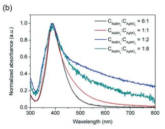
Fig. 6 Effect of NaBH<sub>4</sub>: AgNO<sub>3</sub> concentration ratio on the Ag conversion and size distribution in reactor 1 (60 °C, residence time of 71 s, 0.05 mM AgNO<sub>3</sub>, [NaBH<sub>4</sub>]: [NaOH] = 1:2.75): (a) UV-vis spectra and (b) normalised UV-vis spectra.
