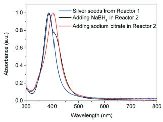
Fig. 8 Normalized UV-vis spectra of silver seeds synthesized in reactor 1 (CFIR; helix diameter: 10 mm, pitch distance:  $1/\pi$  cm, length: 3.2 m, 0.03" ID, residence time: 175 s, 0.05 mM AgNO<sub>3</sub>, 0.025 mM NaBH<sub>4</sub>, and 0.35 mM Na<sub>3</sub>CA, 60 °C) and after growth in reactor 2 (CFIR; helix diameter: 10 mm, pitch distance:  $1/\pi$  cm, length: 3.2 m, 0.03" ID, residence time: 167, 14 mM reducing agents and 2 mM AgNO<sub>3</sub>, 90 °C).
