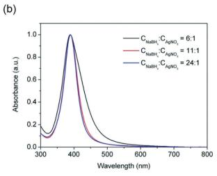
Fig. 2 (a) UV-vis absorbance spectra and (b) normalized absorbance spectra for Ag nanoparticles synthesized with different concentration ratio of NaBH<sub>4</sub>: AgNO<sub>3</sub>. SHR, helix diameter: 10 mm, pitch distance:  $1/\pi$  cm, length: 1 m, 0.03" ID. The total flowrate is 0.5 mL min<sup>-1</sup>, residence time: 54 s.
