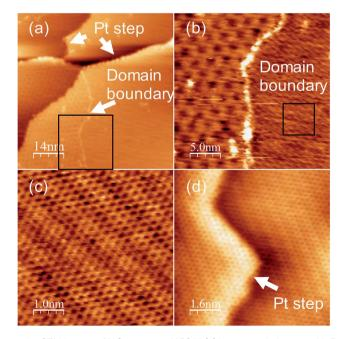
Fig. 2 STM image of NG grown at 1150 K. (a) Large-scale image with Pt (111) step and domain boundary, and (b) magnified image of the rectangle area in (a). (c) Magnified image of the rectangle area in (b). (d) Atomic-resolution image at around a Pt (111) step.
