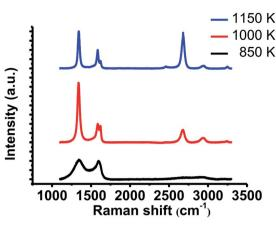
Fig. 3 Raman spectra of the grown films after the transfer onto SiO<sub>2</sub>/Si substrate. All spectra were normalized to the intensity of G band.
