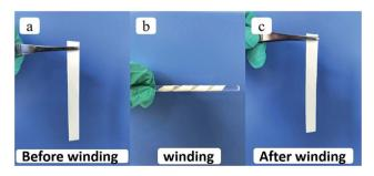
The <sup>29</sup>Si NMR test of precursor hybrid fiber membrane and SF. Fig. 4 Flexibility test of the SF separator before and after winding.
