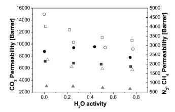
Fig. 1 Permeability (barrer) at different relative humidity ( $T=35\,^{\circ}\text{C}$   $p=1\,$  bar) for the zeolite A/PTMSP MMM (full symbols) and PTMSP membranes (void symbols). N<sub>2</sub> (grey triangles), CH<sub>4</sub> (dark grey squares) and CO<sub>2</sub> (black circles).
