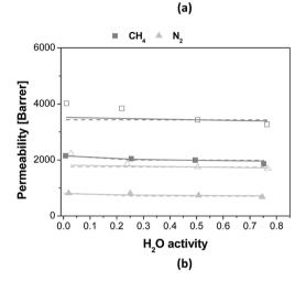
Fig. 7 Permeability of (a)  $CO_2$  (black circles) and (b)  $N_2$  (light grey triangles) and  $CH_4$  (grey squares) as function of water activity for the PTMSP membrane (void symbols) and the zeolite A/PTMSP MMM (full symbols). Dashed lines correspond to the diffusivity-based model and continuous lines to the (diffusivity + solubility)-based model.
