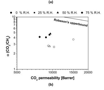
Fig. 3 Comparison of (a) CO<sub>2</sub>/N<sub>2</sub> and (b) CO<sub>2</sub>/CH<sub>4</sub> selectivity as a function of R.H. with the Robeson's upper bound.9 Open symbols: PTMSP. Filled symbols: zeolite A/PTMSP MMM. The symbols indicate the direction towards increasing relative humidity values as follows: 0% (circles) < 25% (squares) < 50% (triangles) < 75% (rhombuses).
