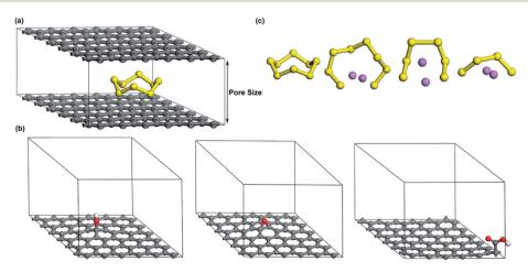
Fig. 1 (a) Microporous graphene (b) microporous structures of hG, eG and cG respectively (c) geometrically optimized minimum energy  $structures of S_8, Li_2S_8, Li_2S_6 \ and \ Li_2S_4 \ respectively \ (carbon, sulfur, oxygen, hydrogen and lithium atoms are represented by grey, yellow, red, white \ (carbon, sulfur, oxygen, hydrogen) \ and \ (carbon, sulfur, oxygen, hyd$ and purple, respectively).
