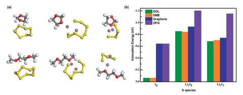
Fig. 8 (a) Interaction of S<sub>8</sub>, Li<sub>2</sub>S<sub>8</sub> and Li<sub>2</sub>S<sub>4</sub> with DOL and DME. (b) Adsorption energies of S<sub>8</sub>, Li<sub>2</sub>S<sub>8</sub> and Li<sub>2</sub>S<sub>4</sub> interacting with DOL, DME, graphene and OFG.
