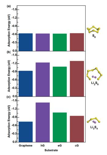
Fig. 3 Adsorption values of (a)  $S_8$ , (b)  $Li_2S_8$ , and (c)  $Li_2S_4$  interacting with graphene, hG, eG and cG.
