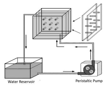
Fig. 9 Schematic showing the apparatus for studying the degradation of scaffolds under conditions of fluid flow.<sup>141</sup> Reprinted with permission from ref. 141 (Copyright © 2007, Trans Tech Publications).
