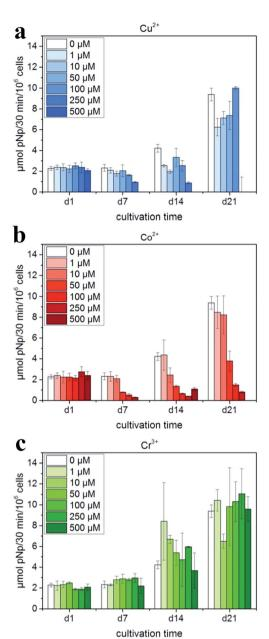
Fig. 7 ALP activity of hMSC cultivated in the presence of Cu<sup>2+</sup>, Co<sup>2+</sup> and Cr3+ ions added to cell culture medium (with OS) in various concentrations: (a)  $Cu^{2+}$ : 0-500  $\mu$ M ( $\mu$ mol  $L^{-1}$ ); (b)  $Co^{2+}$ : 0-500  $\mu$ M; and (c)  $Cr^{3+}$ : 0-500  $\mu M$ . Reprinted with permission from ref. 111 (Copyright © 2017, Elsevier).
