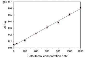
Fig. 3 (a) Differential pulse voltammograms of MIP/GP-PEDOT:PSS/ SPCE recorded in 5 mM K<sub>3</sub>[Fe(CN)<sub>6</sub>]/K<sub>4</sub>[Fe(CN)<sub>6</sub>] after incubation in different concentrations of salbutamol, (b) calibration curve of the MIP/GP-PEDOT:PSS/SPCE. The error bars represent the standard deviation obtained from 6 independent measurements.
