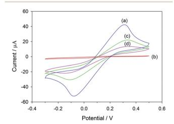
Fig. 1 Cyclic voltammograms of 5 mM  $\rm K_3[Fe(CN)_6]/K_4[Fe(CN)_6]$  in 100 mM KCl at (a) graphene/PEDOT:PSS/SPCE, (b) MIP electrode before template removal, (c) MIP electrode after template removal and (d) MIP electrode after target rebinding.
