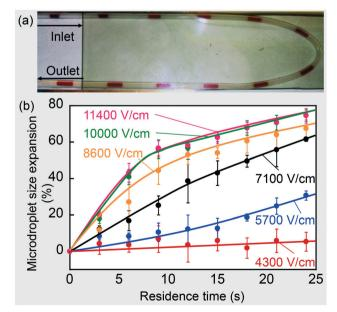
Fig. 2 (a) A photo of the size expansion of the microdroplet train. ITO glass replaced the top copper electrode for optical transparency. (b) Microdroplet size expansion under different field strengths as an indicator of mass transport from the miniemulsion to the microdroplets. Solid lines are added manually to emphasize trends (error bars were obtained with three repetitions and corresponded to a
