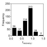
Fig. 2 Distribution of  $f_{\text{recovery},i}$  for spiked chemicals (n=459) in LVSPE. Six chemicals had a  $f_{\text{recovery},i}$  greater than 1.5 (not shown).
