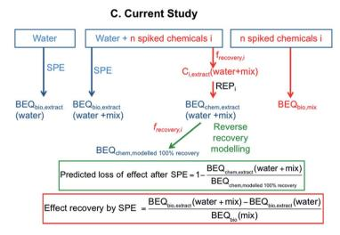
Fig. 1 Overview of approaches commonly used in the literature to evaluate chemical SPE recovery of spiked chemicals expressed as effect (A) and iceberg modelling, which is a comparison of the effect observed in a water sample to the effects predicted for the quantified chemicals (B), with the complementary approach of true effect recovery by SPE applied in the current study (C)
