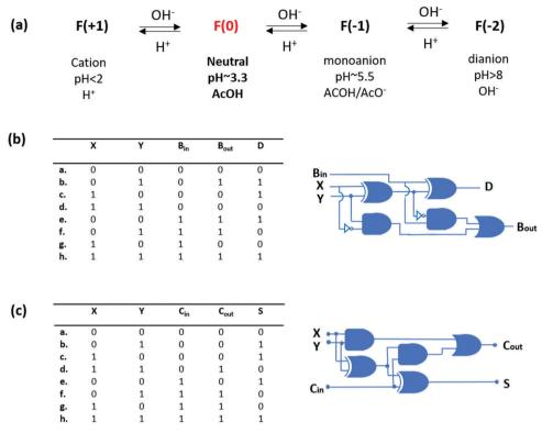
Fig. 6 (a) Different ionization states of fluorescein depending on pH. (b) Truth table for the molecular full-subtractor. (c) Truth table for the molecular full-adder. Reproduced from ref. 9 with permission from American Chemical Society, copyright 2006.
