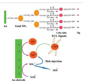
Fig. 7 Schematic illustration of fabrication process (A) and FCI mechanisms (B) of the ECL immunosensor. (Reprinted with permission from ref. 49. Copyright 2008 Elsevier.)
