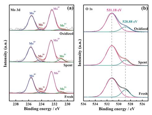
Fig. 9 Mo 3d (a) and O 1s (b) XPS spectra of fresh, spent and oxidized  $La_{5.5}W_{0.6}Mo_{0.4}O_{11.25-\delta}F_{0.05}$  membranes.
