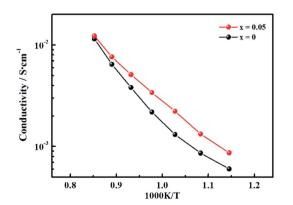
Fig. 6 Conductivity as a function of temperature plotted in the Arrhenius form under a wet (pH $_2$ O = 0.025 atm) 10% hydrogen in argon atmosphere for LWMF $_0$  and LWMF $_{0.05}$  specimens.
