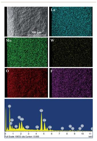
Fig. 3 SEM-EDXS image of the  $La_{5.5}W_{0.6}Mo_{0.4}O_{11.25-\delta}F_{0.05}$  membrane.
