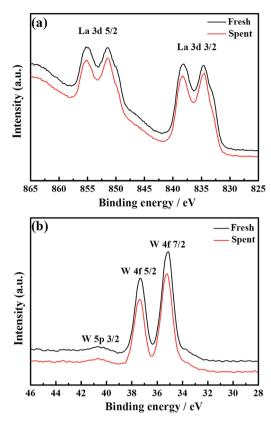
Fig. 8 La 3d (a) and W 4f (b) superimposed XPS spectra of fresh and spent  $La_{5.5}W_{0.6}Mo_{0.4}O_{11.25-\delta}F_{0.05}$  membranes.
