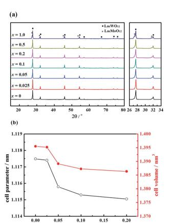
Fig. 1 (a) X-ray diffraction patterns and (b) the cell parameter and the cell volume of the La $_{5.5}$ W $_{0.6}$ Mo $_{0.4}$ O $_{11.25-\delta}$ F $_x$  membranes sintered at 1500 °C.
