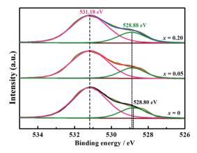
Fig. 4 XPS of O 1s peaks for La<sub>5.5</sub>W<sub>0.6</sub>Mo<sub>0.4</sub>O<sub>11.25- $\delta$ </sub>F<sub>x</sub> (x = 0, 0.05, 0.2) ceramics.
