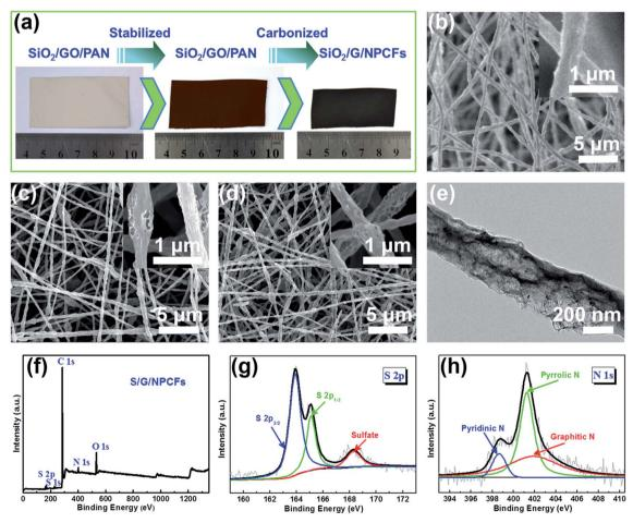
Fig. 1 (a) The photographs of the calcination process of the as-prepared film; (b) typical SEM images of  $GO/SiO_2/PAN$ , (c) G/NPCFs and (d) S/G/NPCFs; (e) TEM image of S/G/NPCFs. (f) XPS spectrum of S/G/NPCFs; high resolution spectra of (g) S/G/NPCFs.
