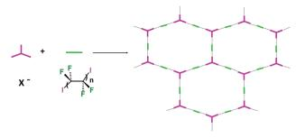
Fig. 3 Schematic representation of the XB driven self-assembly of diiodoperfluoroalkanes 3 with halide anions to form supramolecular anions with (6.3) topology wherein anions are the nodes and dijodoalkanes the sides of the hexagonal frames
