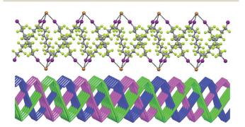
Fig. 5 Top: Partial representation along the crystallographic a-axis (Mercury 3.8, ball and stick) of one undulating honeycomb net in  $1\cdot2e\cdot3d$ . XBs are in black dotted lines. Colour codes as in Fig. 4. Bottom: Schematic view (approximately along the a-axis) of three entangled (6,3) networks in the same compound; three different colours have been used for the three different nets.
