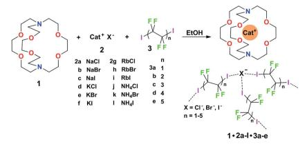
Fig. 2 Starting chemical species 1, 2a-l, and 3a-e and schematic representation of the structural units in corresponding cocrystals 1·2a-l·3a-e. A pattern of three XBs around the anion is depicted as it is the by far most common arrangement in the library (it is present in twenty eight of the thirty one X-ray structures).
