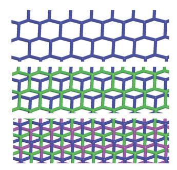
Fig. 6 Superimposition of three honeycomb nets, viewed along the c axis, evidencing their Borromean interpenetration in  $1 \cdot 2e \cdot 3d$ . Top: View of one honeycomb net; mid: a second net (green) is superimposed evidencing that the nets are not interlaced; bottom: the third net (violet) is added and it interlaces the other two as typical for Borromean systems.
